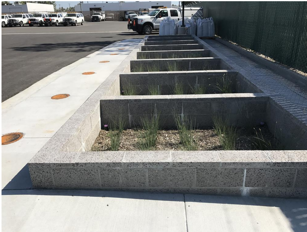
Figure 4-9. Eight identical biofilter test cells (5'x8'x6') built for stormwater research. At the far end of the cells are large bags of biochar supplied by Stanford University researchers that will be used for amending the soil media for pathogen removal experiment.
