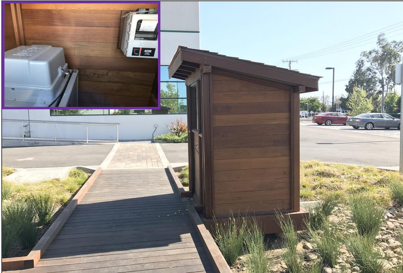
Figure 4-4. Monitoring shed located between Parcels 1 and 2. Inset: the inside of the shed, with ISCO 4230 Bubbler flow meter on the top right and ISCO 6712 FR refrigerated autosampler on the lower left. They monitor continuous flows and take samples at preset intervals from the underground pipe that drains approximately 50% of the entire site.
