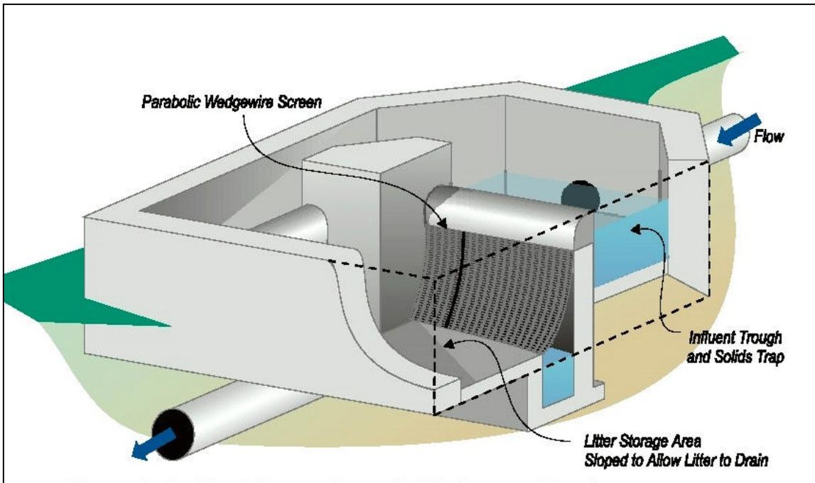
**Figure 3-8 Inclined Screen GSRD**
