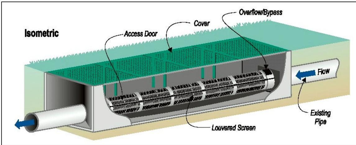
**Figure 3-7 Linear Radial GSRD**
