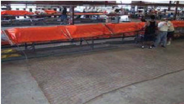
**Figure 3-17 Elastec™ Floating Net Boom**
