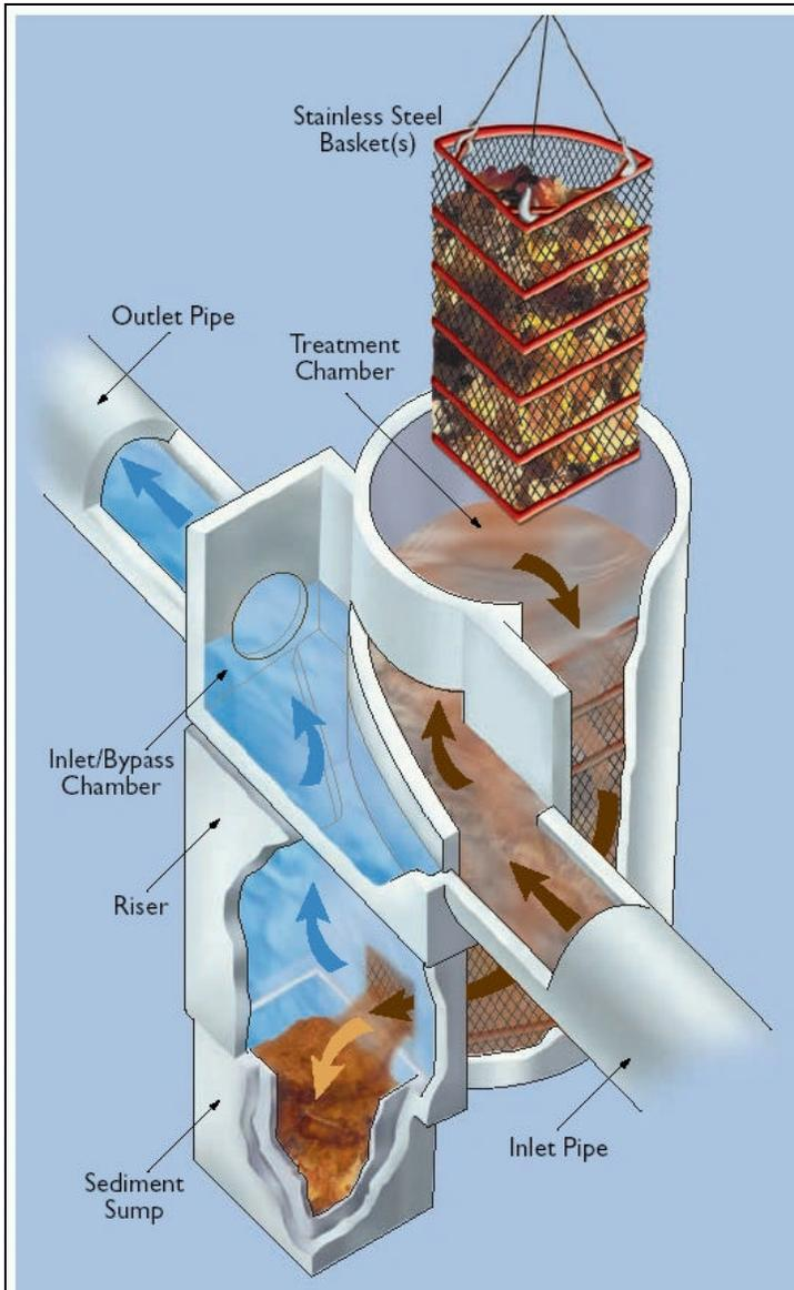
**Figure 3-3 Cleansall™ Gross Pollutant Trap Schematic**
