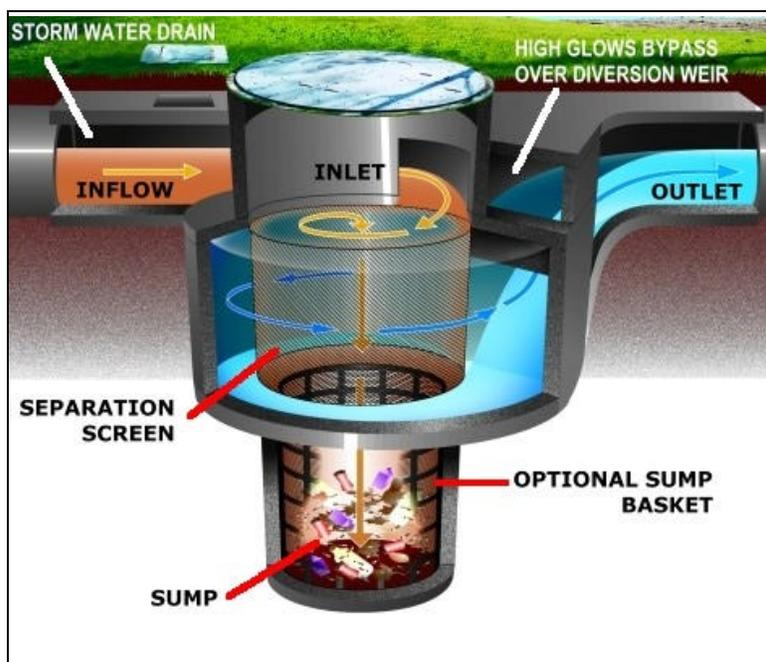
**Figure 3-9 CDS™ Unit Schematic**
