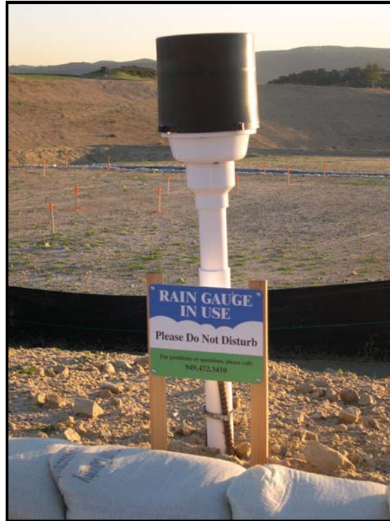
Figure 7. Rain Gauge Setup
