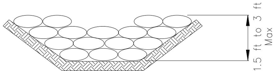
GRAVEL BAG CHECK DAM ELEVATION
